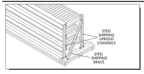
**NOTE**: Carefully examine shipment during uncrating to ensure that essential components are not discarded. This includes guard rail and other necessary hardware.
