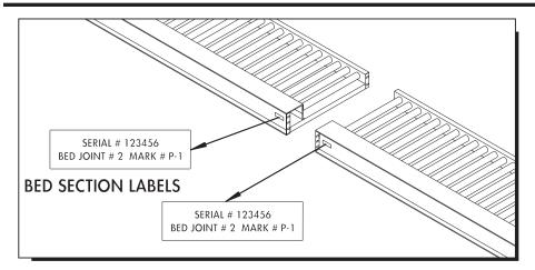
**NOTE:** It is critical for bed sections to be field assembled in proper sequence following bed section labels..
