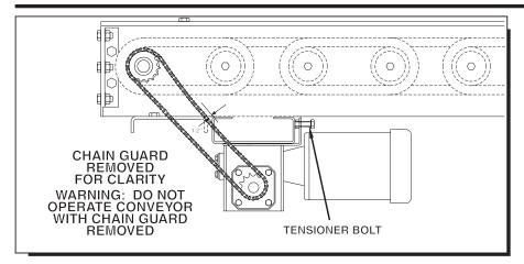
Maintaining proper chain tension is especially important. Again, a periodic visual inspection is recommended to ensure chain tension within a pre-determined operating range.
