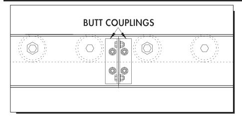
**NOTE:** During unit installation, take diagonal measurement across unit and make adjustments as necessary to square unit prior to final assembly of supports
