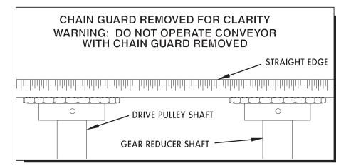
Set up and maintenance of drive sprocket and drive chain alignment is critical. A periodic visual inspection is recommended to confirm alignment of drive components (which includes both drive sprockets and drive chain). Should set screws become loose, drive sprockets are subject to excessive wear and ultimately, to untimely replacement.
