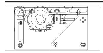
Always leave popout roller (see illustration at left) in place when permanently attaching any gravity conveyor to power conveyor. Never connect powered belt conveyors directly to gravity conveyors without using the pop out roller.
