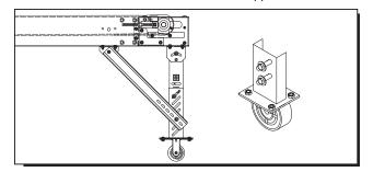
Knee braces are most commonly used at the terminal ends of long runs of conveyor lines and are recommended on inclined (or declined) floor-to-floor belt conveyors for added stability.
