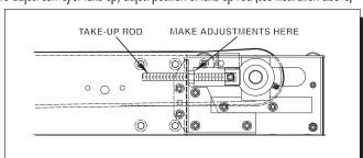
as required. Remember to equally adjust both sides to hold take-up pulley square (to maintain unit squareness for belt tracking). Operating unit with slipping belt will decrease life of both belting and pulley lagging.
