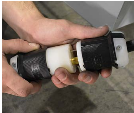
Align the connector blades with the plug inlets.
