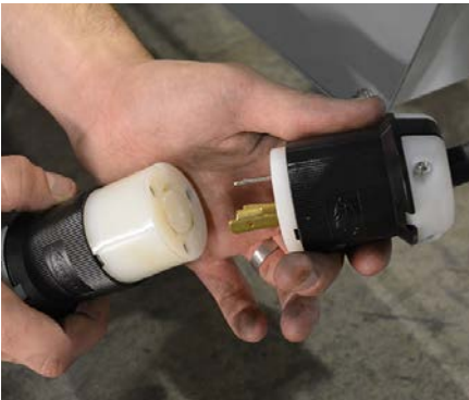
Align the connector blades with the plug inlets.
